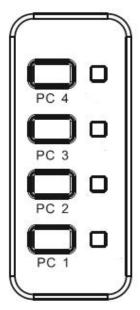
Buttons on panel are selection buttons. Just press one button and then you can select the corresponding port. Each button has upper and lower two LEDs indicating on line and selected status. The upper indicates the on line status. It lights if the corresponding computer is on line. The lower indicates the selected status. Since there is only one port selected at one time, the only one LED lights to show that the corresponding computer is selected.
